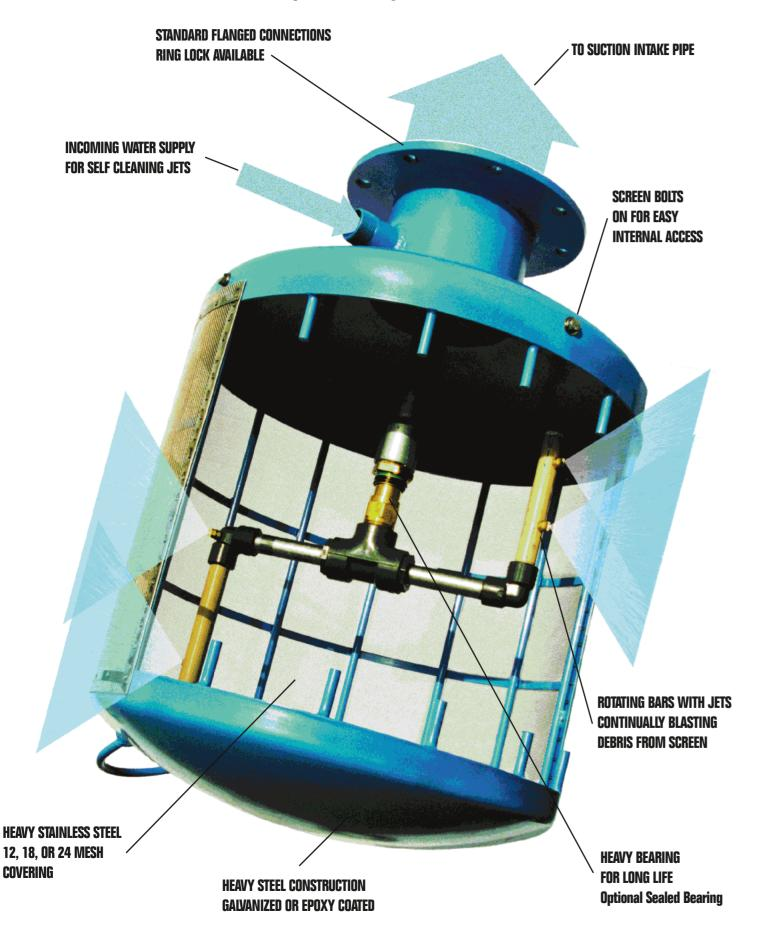
If you irrigate, you know how important it is to keep equipment running smoothly and water flowing freely. Whether you are pumping water from a stream, canal, river, irrigation ditch, pit or sump, or a golf course pond, you need the water to be free of trash and debris that could block water flow and damage the pump or clog water-distribution equipment. Call factory for advice in waste treatment and manure lagoon usage.
